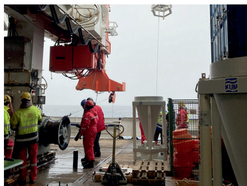
Deployment of long-term sediment traps as part of long-term moorings in Fram Strait.
